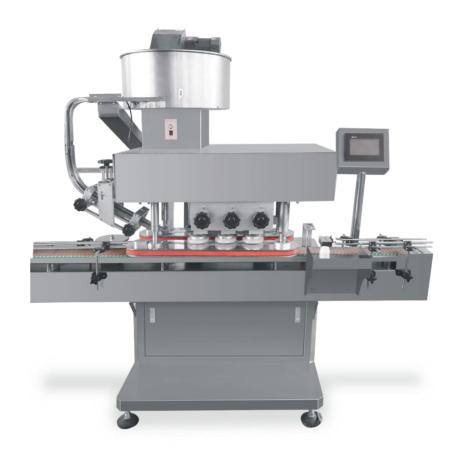
The bottle caps neatened by the cap neatening device ,the bottle caps with mouth up are carried to the caps collecting guideway,the bottles come from other equipment of the assembly line enter the caps collecting area. The bottles move ahead with clamping of the two sides clamping device then the caps match the bottles automatically.
