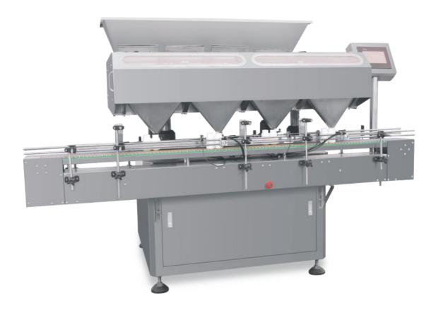
The block bottle device on the passing bottle-track of the conveying bottle system make the bottles which came from the previous equipment stay in the bottling position ,waiting to be filled in .The medicine goes into the medicine container in order by the vibration of the feeding corrugated plate.
