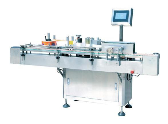
The bottles which are needed labelling transfer by the bottle carrying guideway separate at the same distance by the bottle distance adjustment device, the photoelectric sensor can feel the bottles passing by and send out the signal.
