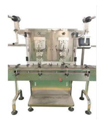
The block bottle air cylinder on the passing bottle-track of the conveying bottle system make the bottles which came from the previous equipment stay in the drying agent filling position ,waiting to be filled in the drying agent .The bottle mouth faces to the clipping system correctly .
