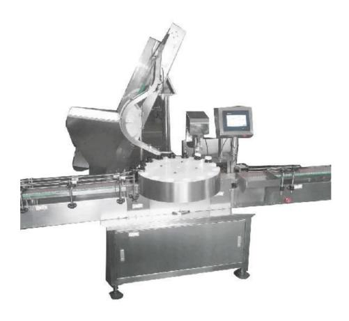
Its function automatically completes bottle delivery, filling, upper cover, rotating cover and so on. The utility model has the advantages of simple structure, stable action, and can solve the positioning and filling problems of the special-shaped bottle.
