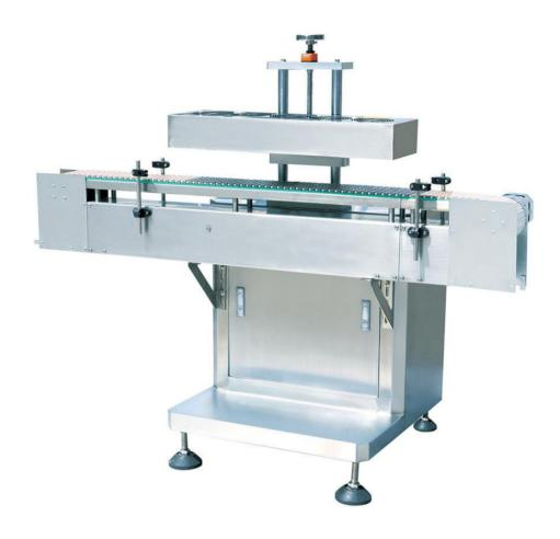
The bottles with aluminium foil pass under the inductive head, the aluminium foil heats after receiving the energy produced by the inductive head.
